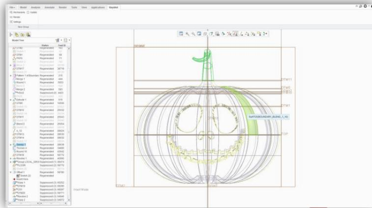
First I created a CAD model using CREO 2.0 surface modeling. The face was created using a Google image which I converted to a vector image in Illustrator and then exported as dxf after which I could use it as a feature in CREO!
