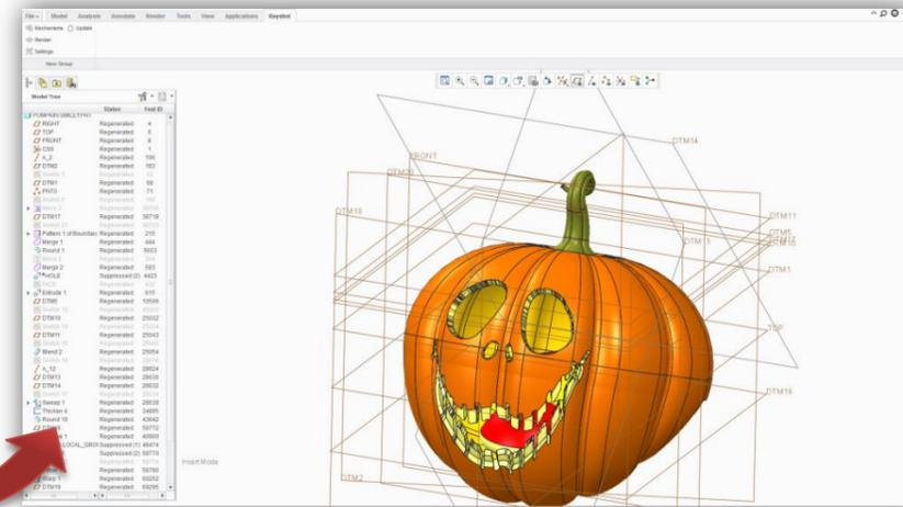
After being satisfied with the static model, I created a feature called "warp" which allows me to stretch geometry by simply filling in an angle. I then simply pressed the render button of the Keyshot-plugin after which the CREO model is loaded in Keyshot.
